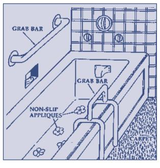
straight downward movement of the arms. In contrast, wall mounted grab bars offer less support because the older adult must reach to the side and bend forward during the transfer process to grab the bar losing the benefit of a downward thrust offered by the double armrest system. As additional cautionary measures, adhere non-slip adhesive strips in a non-contrasting color to the floor in front of the toilet to secure client footing during transfer, only use bathroom rugs with nonskid backing,
